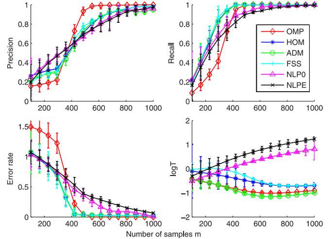
Fig. 1. Comparison of the six algorithms with fixed  $n = 1000$  and  $k = 100$ . The curves show the average over 50 trials and the error bars show the standard deviation.
