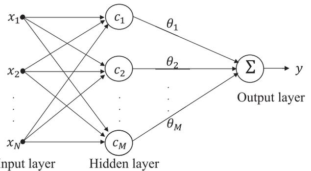
Fig. 4. Structure of the RBF network with a single output neuron.
