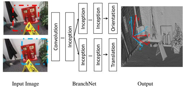
Fig. 1. Multi-task CNN for camera relocalization. Given an input image, the CNN predicts the 6-DOF of the camera. A new orientation representation Euler6 is employed. Both data and label are augmented by a method named pose synthesis, which gives different label to different patches extracted from the input image.
