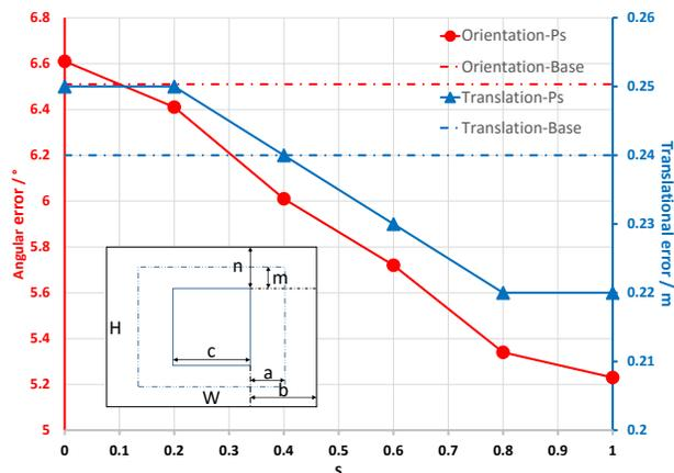
Fig. 6. Median results of PoseNet-Euler6 with different range factor  $s$  on the Chess scene. The inset shows the location of extracted patch in the image, specified by  $s$ , which is defined as  $s = \frac{a}{b} = \frac{m}{n}$ . The black rectangle is the image, the solid blue square is the central patch of the image. The dashed rectangle denotes the area in which the patch can be extracted.
