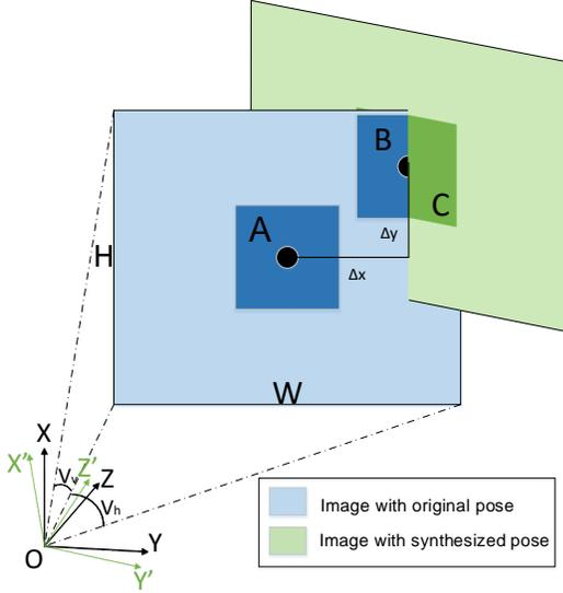
Fig. 4. Pose synthesis. OXYZ and OX'Y'Z' are coordinate systems of original camera  $c$  and rotated camera  $c'$ . Patch A and patch C are central patches of images captured by  $c$  and  $c'$ . Patch B has tiny difference with C so that the new pose OX'Y'Z' can be synthesized.
