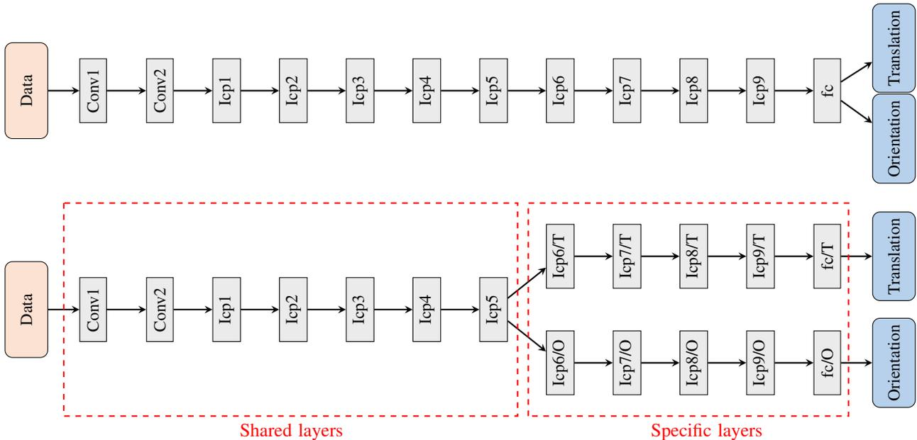
Fig. 2. PoseNet and BranchNet. **Top:** Architecture of PoseNet in which orientation and translation vectors are predicted by the same fully connected layer. **Bottom:** Architecture of BranchNet. The orientation and translation vectors are predicted by different branches. The “Icp” means “Inception” module of GoogLeNet.
