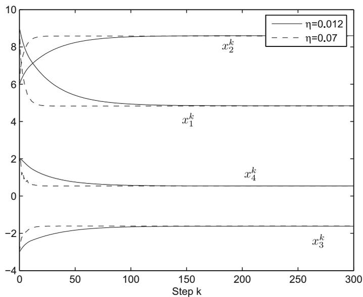
Fig. 3. Transient behavior of the discrete-time dynamic system (11) for solving the problem in Example 1 with different step sizes from the same initial point.
