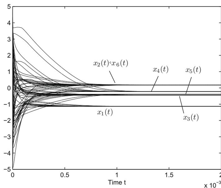
Fig. 5. Transient behavior of the continuous-time dynamic system (10) from 10 random initial points for solving the second problem in Example 2.
