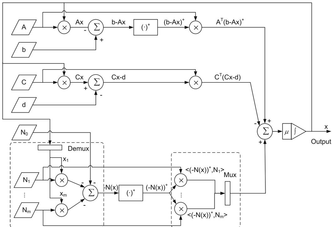
**Fig. 1.** Block diagram of the neural network for realizing continuous-time dynamic system (10). In the left dashed rectangle, the vector  $x$  is decomposed to components, while in the right dashed rectangle, some scalars join together to constitute a vector.
